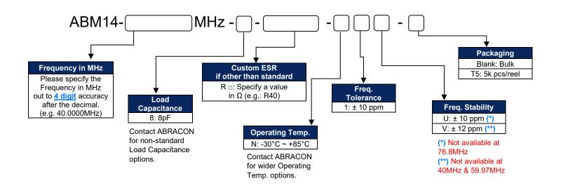
Note 3: Contact Abracon for part number requests with carrier frequency callouts up to 5 & 6 digit accuracy after the decimal.
