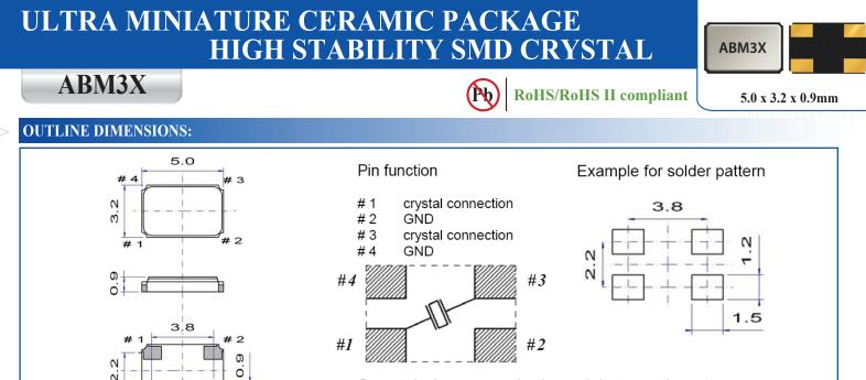
Do not design any conductive path between the pattern
